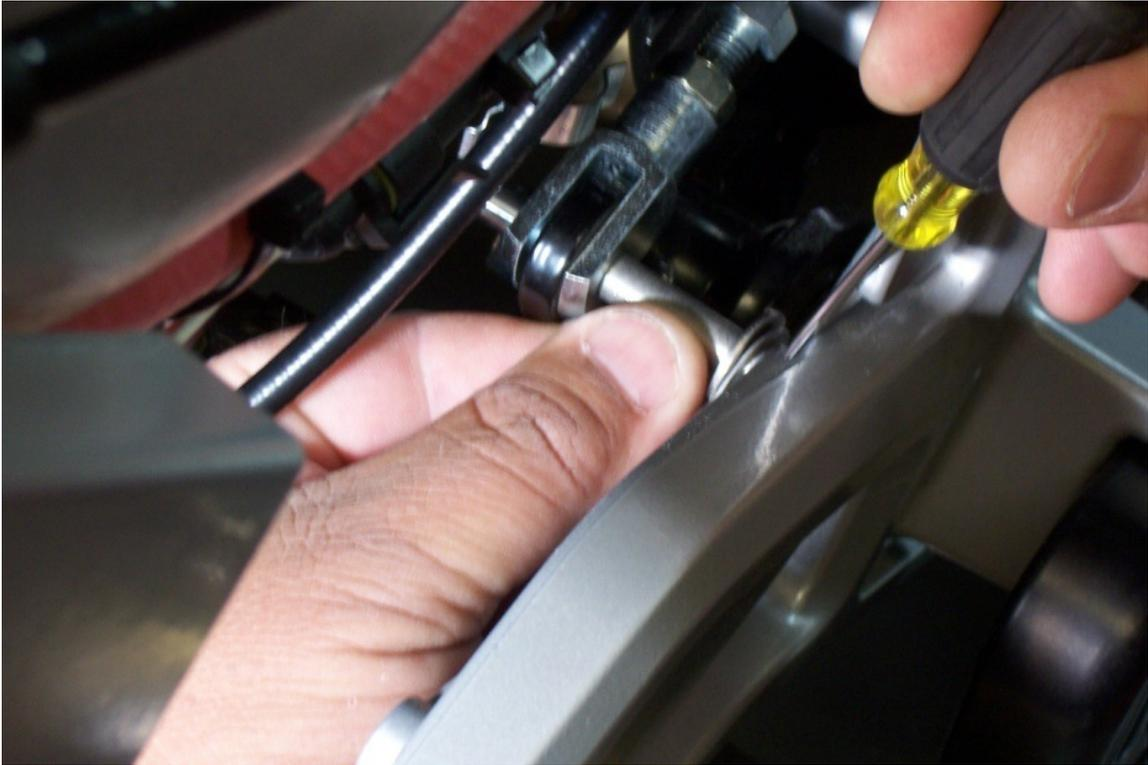
7. Install Washer then insert Rue Ring Cotter into Clevis Pin. Move the washer against the Rue Ring Cotter and center the Clevis Pin so that there is equal spacing between the head of the Clevis Pin and Washers and the OEM Clevis.
