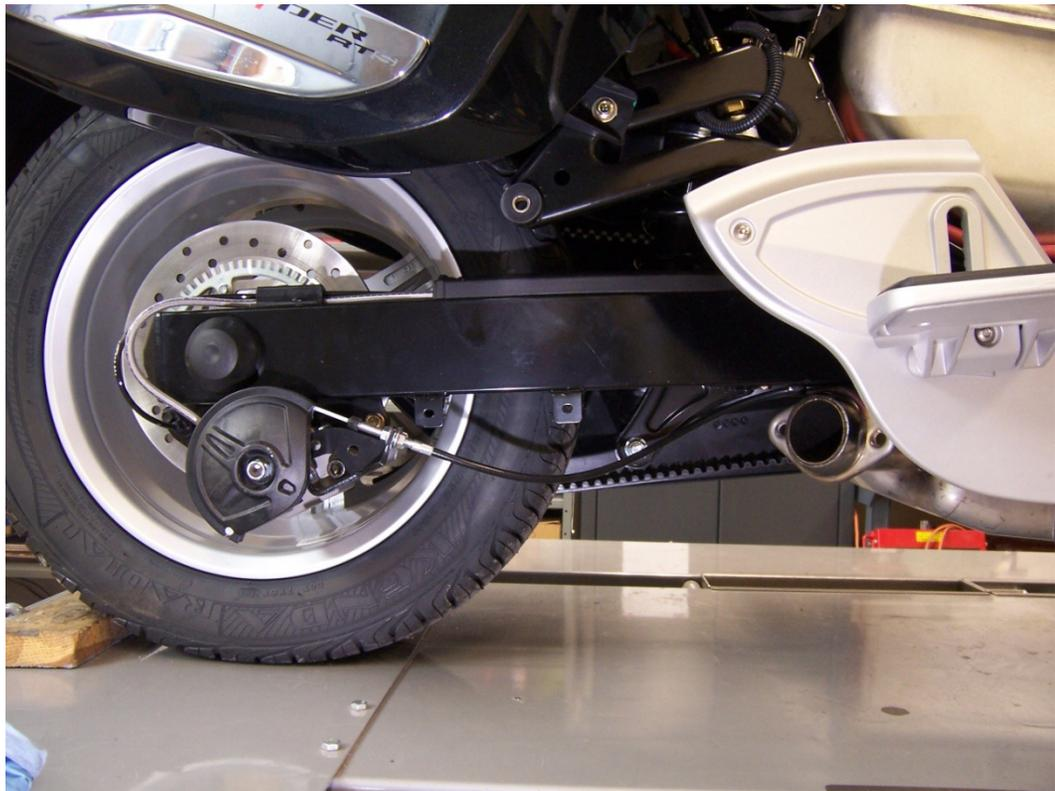
9. Bolt brake line to the Slave Cylinder with the Bleeder Banjo Bolt and 2 Crush Washers. Bring bracket and slave assembly underneath the Spyder so that the holes in the bracket line up with the holes in the top of the Driver's Footrest Support and the new clevis straddles the OEM clevis as shown below. **Note: The picture below is showing the 2010 model being installed but the process is still the same.**
