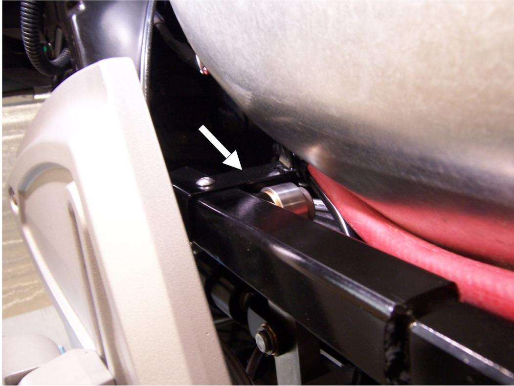
13. Route Braided Brake Line from Slave Cylinder to the Handle Bar as shown in the following pictures. Remove right hand lower Handle Bar Cover.
