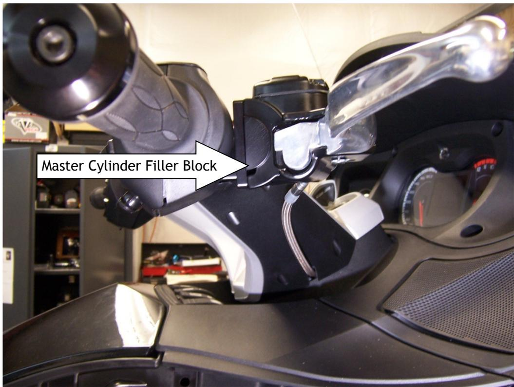
17. Attach Master Cylinder Bracket to Accessory Bracket using 5/16"-18 x 3/4" Flathead Screw.
