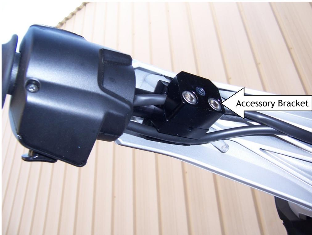
16. Attach Master Cylinder Bracket to the Master Cylinder using 2 1/4"-20 x 5/8" Flathead Screws as shown below with Master Cylinder Filler Block in between.
