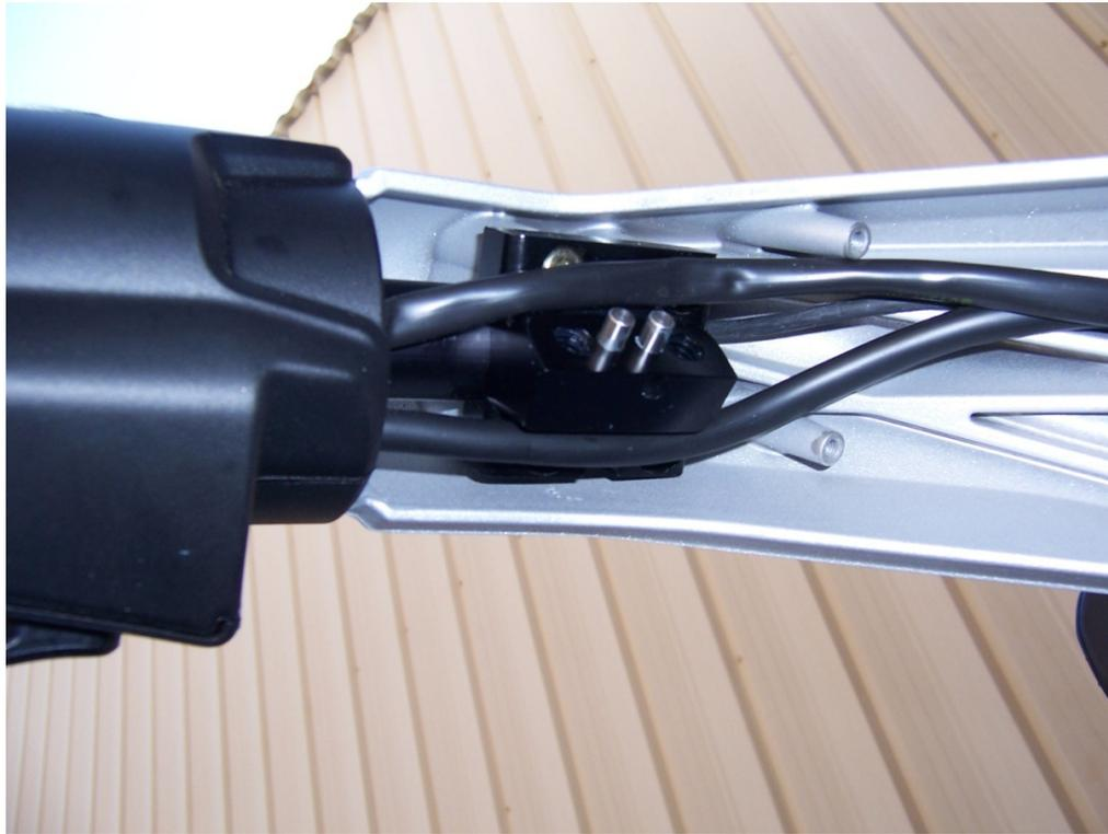
15. At this time the Lower Handlebar Cover would be installed and then the Accessory Bracket. The following picture shows the Accessory Bracket mounted without the cover in place. Be sure not to pinch the wire bundle when installing.
