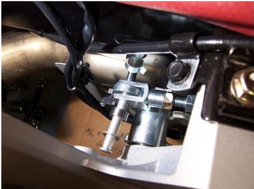
7. Install 1/4" bushing and washer then insert the Rue Ring Cotter into Clevis Pin. Locate the bushings against the OEM clevis and position the Clevis Pin so that there is 1/4" spacing between the washers and the bushings.
