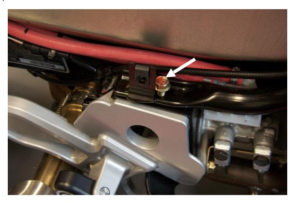
4. Remove the Cotter Pin and unhook the Hook Lock from the Clevis on the Master Cylinder Rod. DO NOT REMOVE THE PIN FROM THE CLEVIS AT THIS TIME!! **NOTE: The following picture does not show the Cotter Pin that must be removed.**
