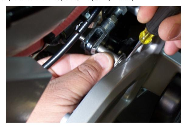
7. Install Washer then insert Rue Ring Cotter into Clevis Pin. Move the washer against the Rue Ring Cotter and center the Clevis Pin so that there is equal spacing between the head of the Clevis Pin and Washers and the OEM Clevis.
