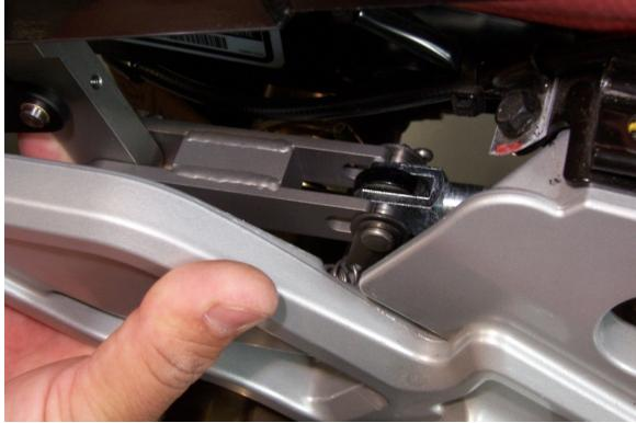
9. Install two M8x40mm Hex Head Bolts through the bracket and into the top of the Driver's Footrest Support where the 2 socket head screws are shown in the picture.
