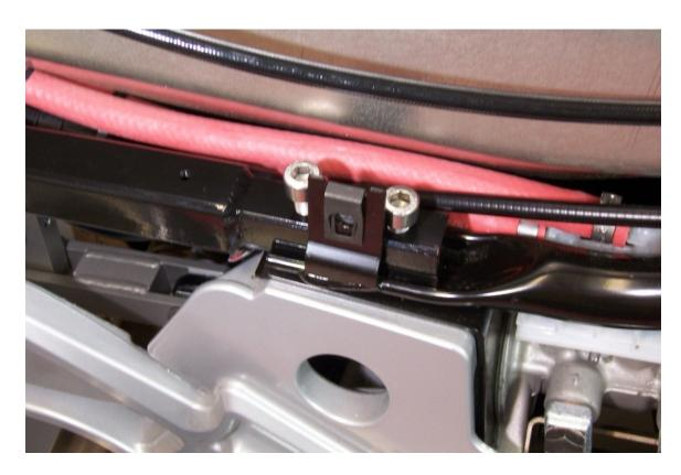
10. Install Master Cylinder to handle bars as shown.
