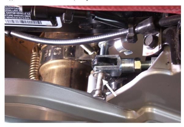
6. The use of a small screwdriver to help push the pin into place maybe necessary.
