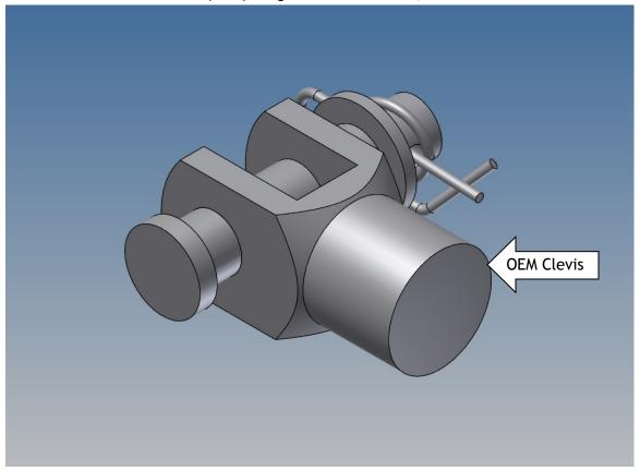
8. Bring bracket and slave assembly underneath the Spyder so that the holes in the bracket line up with the holes in the top of the Driver's Footrest Support and the new clevis straddles the OEM clevis as shown below.
