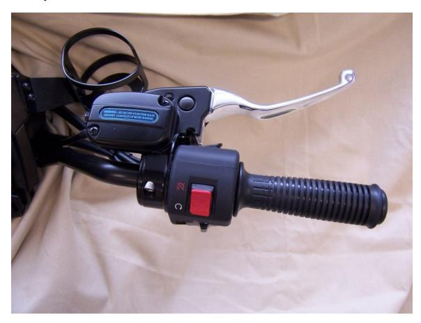
11. Route Braided Brake Line from Master Cylinder to Slave Cylinder as shown in the following pictures. An alternate route can also be used by routing from the master cylinder to the left side of the Spyder and along the side of the air box then routing through the area between the air box and the fuel tank to the right side.
