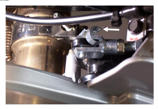
5. Use the supplied Clevis Pin (Item #19) to start pushing the OEM Clevis Pin out.
