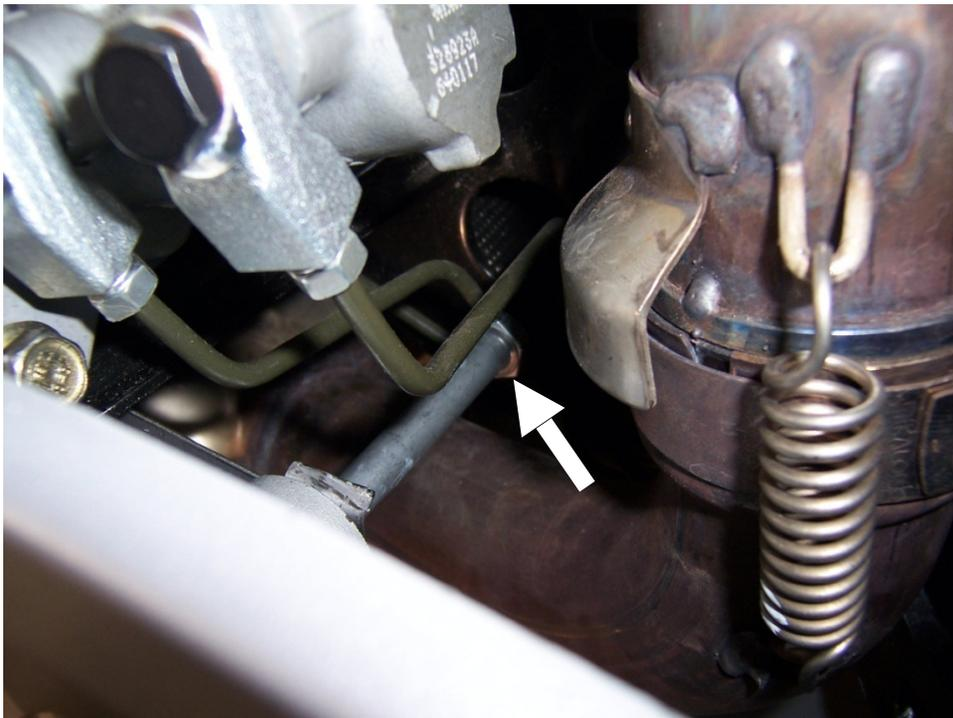
7. You should be able to remove the the Brake Lever. There are two washer/spacers on both sides of the bearings on the Brake Lever. Do not lose these. One is shown here.
