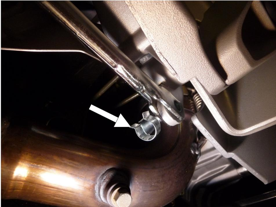
5. On the right side underneath the Footrest there is a nut on the bolt that the Brake Lever pivots on. This bolt also holds the Footrest to the Footrest Support Casting. The head of this bolt has a sheet metal retaining tab that needs to be bent up to get a wrench on the bolt head. Remove the nut and washer.
