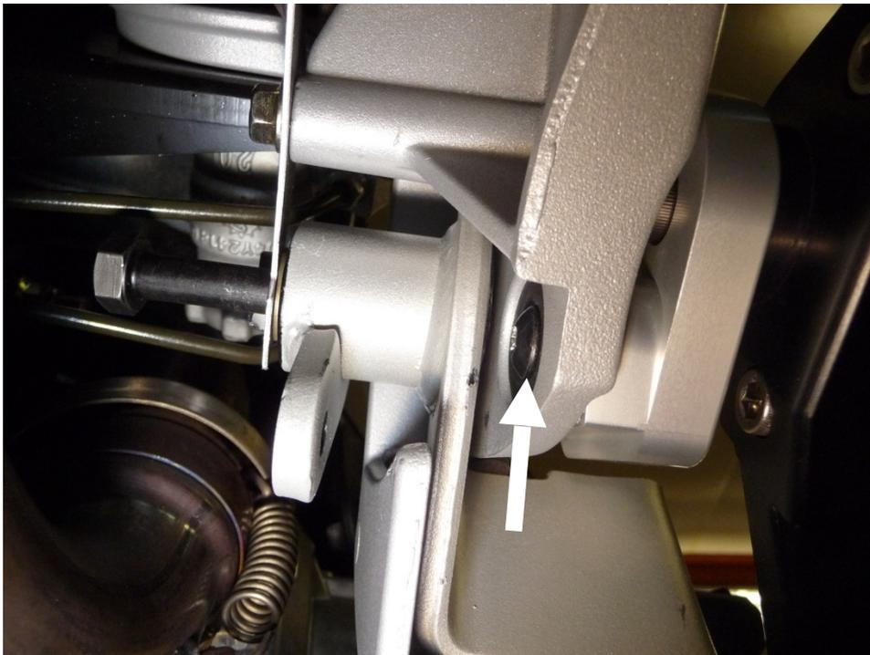
9. The left hand side is easier. Remove the weight and the rubber top from the Footrest. Remove the nut and bolt going through the Footrest and the Footrest Support Casting. Then the button head screw from the inside of the Footrest Support Casting.
