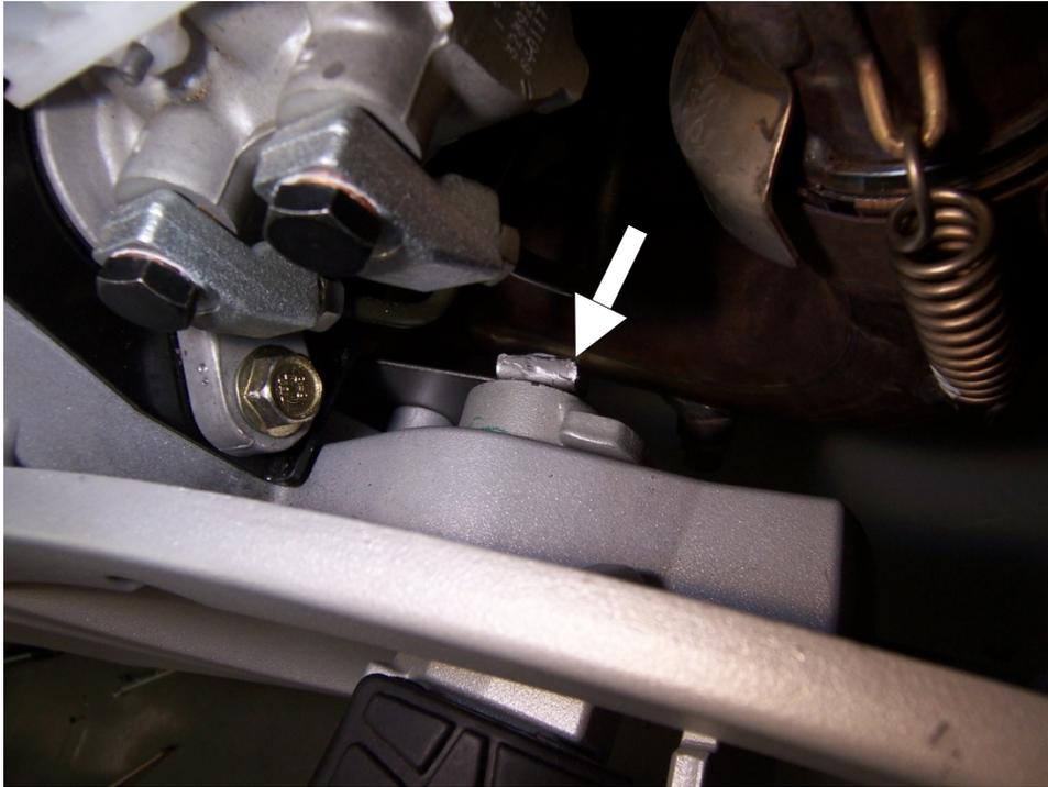
6. This same bolt is quite long and when trying to remove it the head of the bolt might hit one of the brake lines. Gently push the brake line over to one side to allow the head to go past the brake line and remove the bolt.
