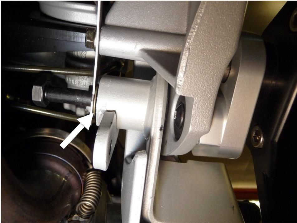
8. On the inside of the Footrest Support Casting there is a 6mm Button Head Screw with a Torx drive that needs to be removed. The Brake Lever was removed in order to access this screw. Footrest will come off when this screw is removed.
