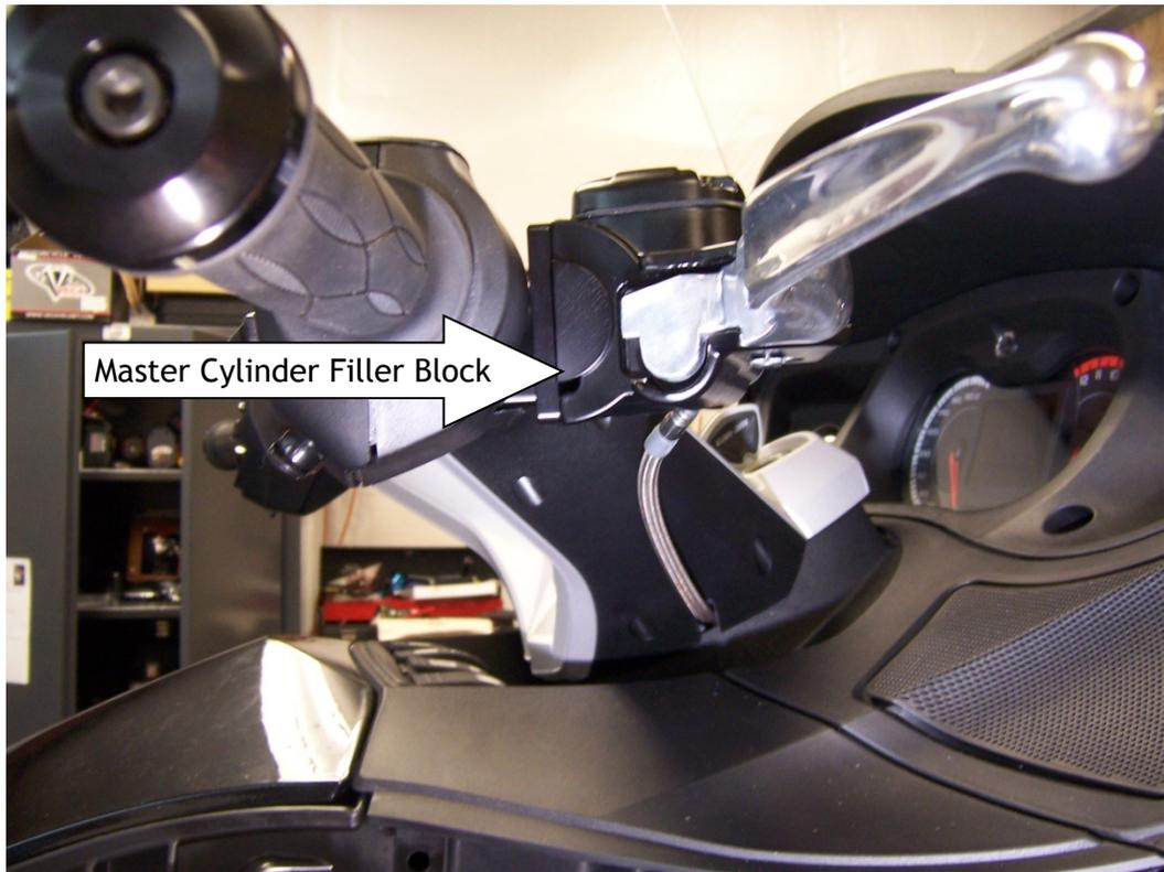
17. Attach Master Cylinder Bracket to Accessory Bracket using  $5/16''-18 \times 3/4''$  Flathead Screw.
