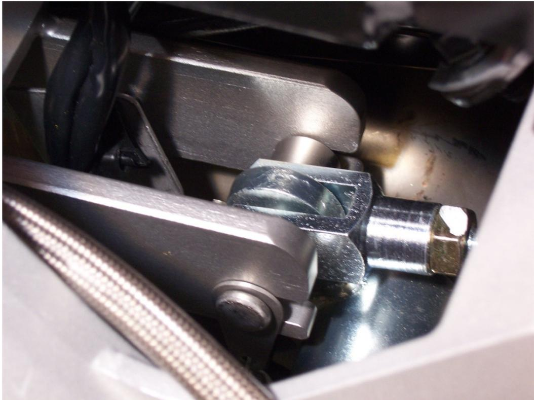
10. Install two M8x40mm Hex Head Bolts through the bracket and into the top of the Driver's Footrest Support.
