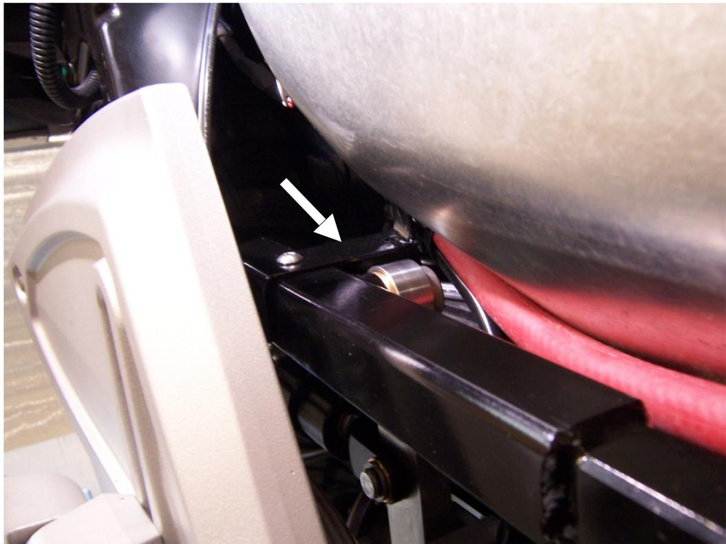
12. Pull back Spring and Link Washer and attach to Clevis Pin at the rear of the Slave Cylinder. Install Cotter Pin and then spread apart to retain.
