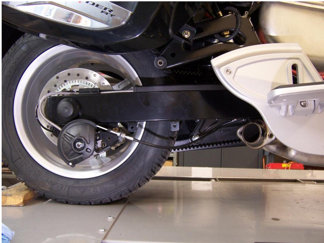
9. Bolt brake line to the Slave Cylinder with the Bleeder Banjo Bolt and 2 Crush Washers. Bring bracket and slave assembly underneath the Spyder so that the holes in the bracket line up with the holes in the top of the Driver's Footrest Support and the new clevis straddles the OEM clevis as shown below. Note: There is no cotter pin in this clevis pin at this point at arrow "A"
