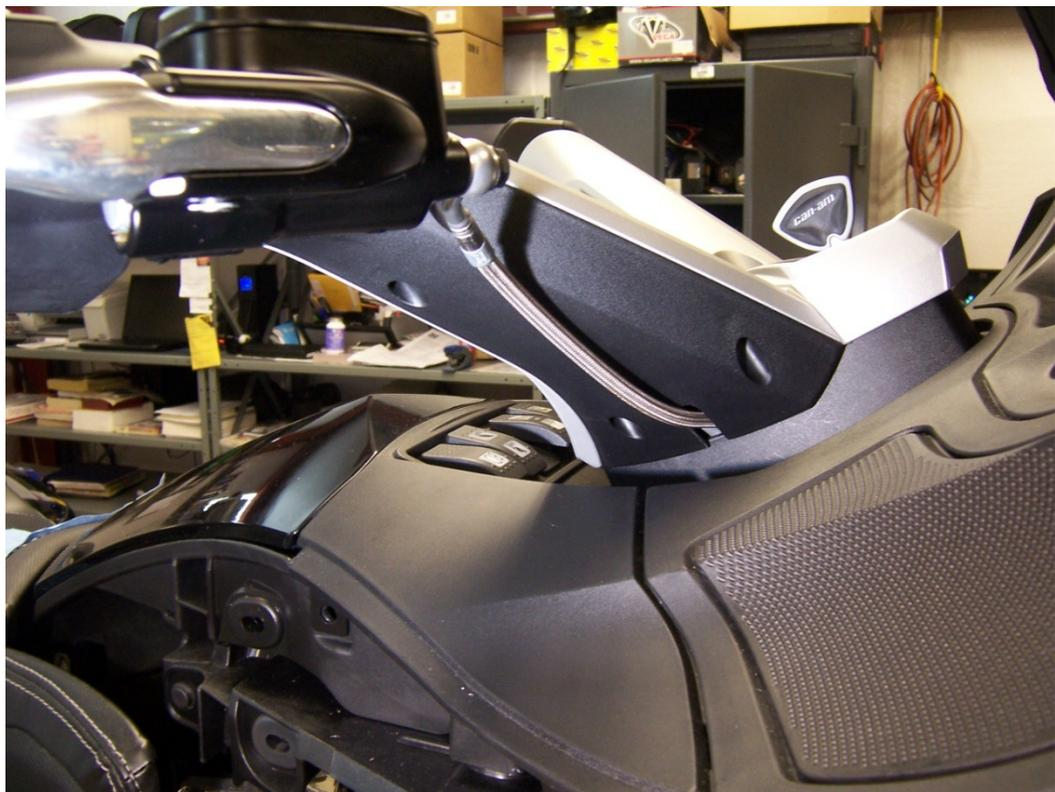
19. Attach brake line to the master cylinder using the supplied black banjo bolt and two crush washers. Fill master cylinder with DOT 4 brake fluid and bleed till there is no air coming out of the bleeder valve. Connecting a clear tube to the bleeder will help from making a mess and you can easily see when there is no more air coming from the slave cylinder.
