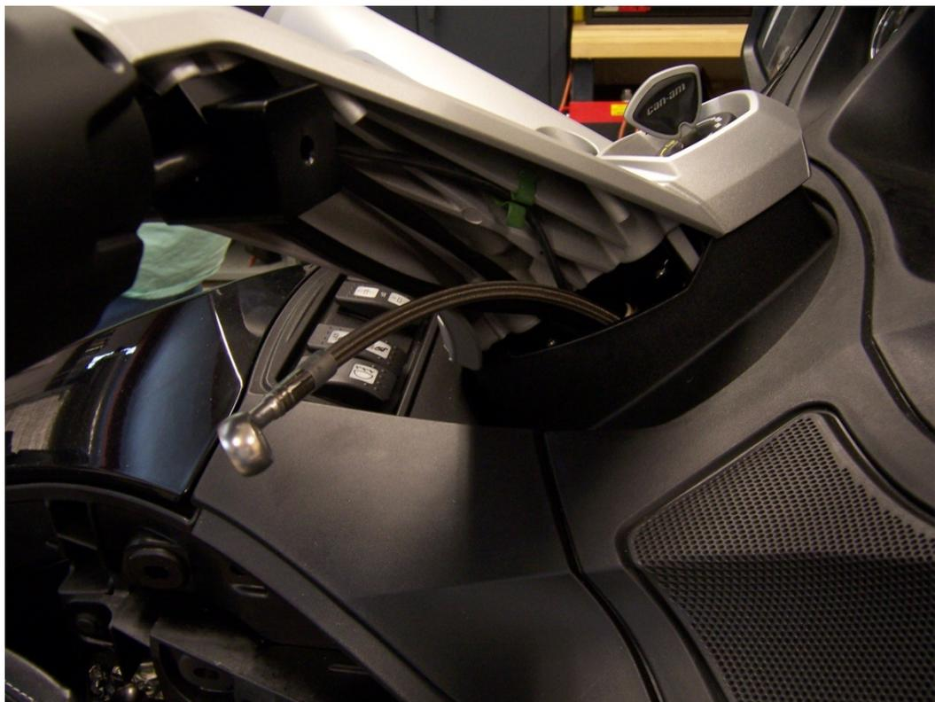
14. Remove 4 screws holding the throttle clamp and replace with the one as shown below. Notice the placement of the wire bundles on either side of the mounting boss. Place the the 2 3/16" x 1/2" dowels as shown.
