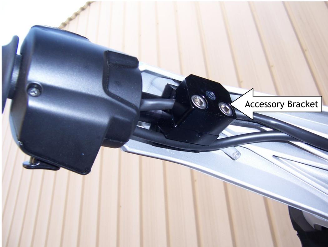
16. Attach Master Cylinder Bracket to the Master Cylinder using 2  $\frac{1}{4}$ "-20 x  $\frac{5}{8}$ " Flathead Screws as shown below with Master Cylinder Filler Block in between.
