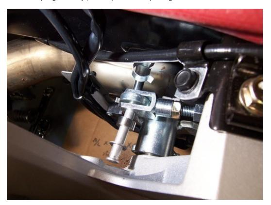
7. Install 1/4" bushing and washer then insert the Rue Ring Cotter into Clevis Pin. Locate the bushings against the OEM clevis and position the Clevis Pin so that there is ¼" spacing between the washers and the bushings.
