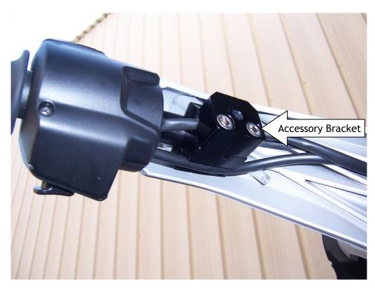
16. Attach Master Cylinder Bracket to the Master Cylinder using 2 ¼"-20 x 5/8" Flathead Screws as shown below with Master Cylinder Filler Block in between.
