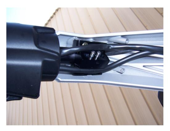
15. At this time the Lower Handlebar Cover would be installed and then the Accessory Bracket. The following picture shows the Accessory Bracket mounted without the cover in place. Be sure not to pinch the wire bundle when installing.
