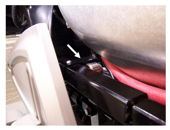
13. Route Braided Brake Line from Slave Cylinder to the Handle Bar as shown in the following pictures. Remove right hand lower Handle Bar Cover.
