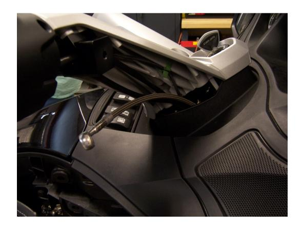
14. Remove 4 screws holding the throttle clamp and replace with the one as shown below. Notice the placement of the wire bundles on either side of the mounting boss. Place the the 2 3/16" x ½" dowels as shown. **Note: The picture** below is showing the installation on the 2010 model being installed but the process is still the same.
