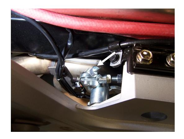
6. Use the Clevis Pin and Spring Assembly from Step #4 to start pushing the OEM Clevis Pin out.
