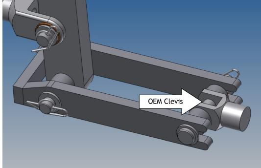
10. **The top picture is showing the 2010 model**. The bottom picture shows the Brake Actuating Clevis along with the spacers for the 2013 model and how it looks when installed onto the OEM Clevis.
