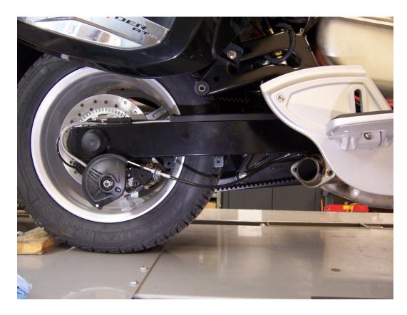
9. Bolt brake line to the Slave Cylinder with the Bleeder Banjo Bolt and 2 Crush Washers. Bring bracket and slave assembly underneath the Spyder so that the holes in the bracket line up with the holes in the top of the Driver's Footrest Support and the new clevis straddles the OEM clevis as shown below. **Note: The picture below is showing the 2010 model being installed but the process is still the same.**
